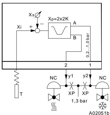
For heating and cooling: use NC valves
