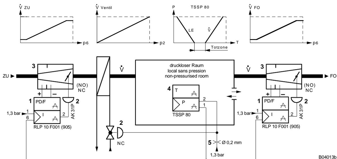
5. Control facility for variable air volume, with re-heater, for 'open rooms'; normally-open re-heater; room-temperature controller has control action A.
